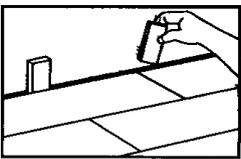
6. Remove the wedges after installation
